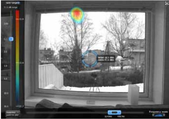
This same procedure with omnidirectional loudspeaker on the outside of the facade emitting white noise, and the acoustic camera on the inside filming an area of interest, could be used on other walls and windows as well. As seen below on a different window and wall, again the main source contribution is visualized as being the air valve above the window.
