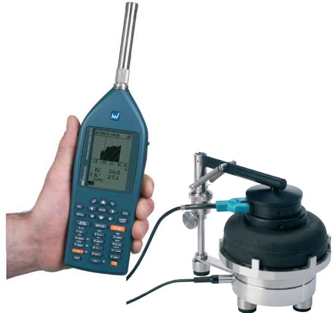
Nor140 Sound Analyser and Artificial Ear Type 43AA
